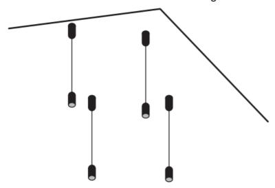
2. Thread the cables through the holders and attach them to the LED panel.
