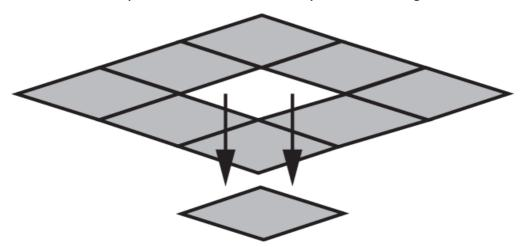
2. Insert the LED panel into the ceiling and connect the driver to the power supply L (brown), N (blue).
