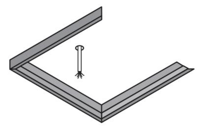
2. Then, insert the LED panel into the frame and connect the driver to the power supply L (brown), N (blue).
