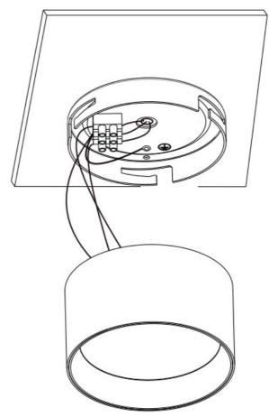
4. Place the light fixture onto the ceiling bracket.
