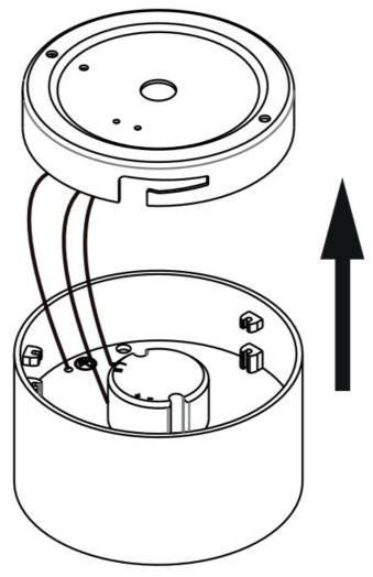
5. Secure the light fixture to the ceiling bracket by turning it.
