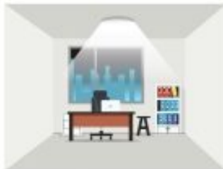
2. With insufficient ambient light, the sensor turns on the light when motion is detected.
