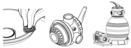
Remove the funnel and clean the edge of the container opening carefully, and residues. To facilitate the start-up, it is recommended to fill the sand filter tank to ¾ with water. Then mount the 4-way valve and the filter gasket. The connection is made with a clamping ring. The clamping ring is screwed to the clamping ring screw and clamping ring nut.
