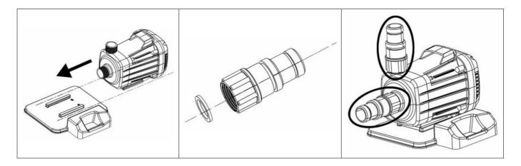
Install the drain plug. Screw the internal filter together in the direction of the arrow as shown. Then assemble the outer connection piece and the internal filter and finally install them with the tank.
