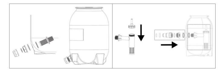
Fill the enclosed filter balls into the tank. Insert the base of the tank into the recess in the pump plate. Make sure that the drain plug is pointing outwards.
