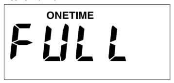
Indicates that the logging capacity (16,000 readings\*) has been reached in One Time mode, and recording has been stopped.
