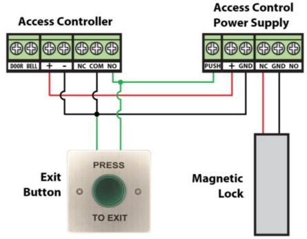
This example shows a "Fail-safe" scenario. When the "Press to Exit" button is pressed the access control power supply then releases power from the lock, and if power is lost then the lock also releases.
