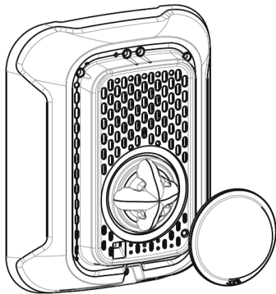
FIGURE 1. COLOR LENS INSTALLATION TO LED WALL MOUNT DEVICE
