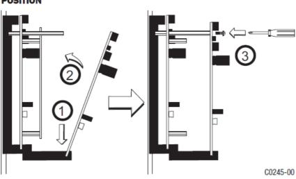
FIGURE 6B. INSTALLATION OF CR-6A MODULE IN FRONT CHASSIS POSITION
