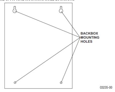
FIGURE 3. TYPICAL MOUNTING HOLE LOCATIONS
