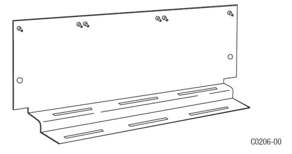
The BB-2A cabinet has a built-in chassis that will accommodate one or two CR-6A modules. (See Figure 2.)
