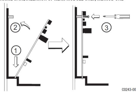
FIGURE 5. INSTALLATION OF REAR MODULE ONLY, METHOD ONE
