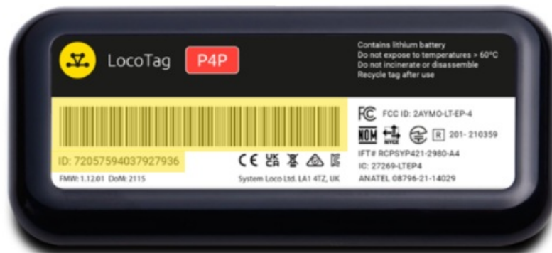
Fig 2. An image of the LocoTag P4P with the device ID and barcode highlighted.
