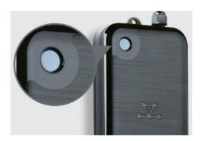
! The button and LED light are on the face of the device in the top-left corner
