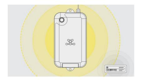
Any activated LocoTag or LocoTrack configured as a Tag will begin reporting through the switched on LocoTrack HFR4 as soon as they come into range, 20m (65.6ft) indoors and 80m (262.5ft) outdoors.
