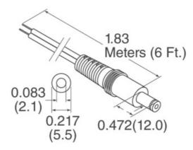
(!) 5V power supply unit should be sourced from a reputable supplier with a standard 2.1mm Barrel Jack (2.1×5.5)
