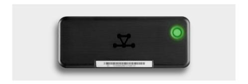
The all-in-one Power Button/LED/Light Sensor are on the face of the device in the top-right corner
