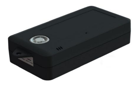
Our C2PL LocoTags have been developed to work alongside the LocoTrack tracking and monitoring devices. They can report presence / absence as well as data for alert notifications (temperature & proximity). The logging function checks and stores temperatures every 60 seconds to local memory.
