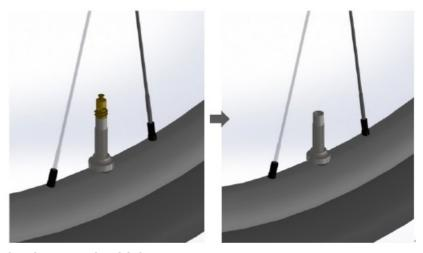
2. Insert the TPMS body onto the Valve.
