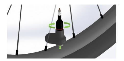
7. When the TPMS is about to contact the bottom surface, adjust the direction of the TPMS and hold it in place with one hand, then use the other hand to continue tightening the adaptor until it is finger-tight. \* (Make sure the upper O-ring is fully sunk into the TPMS and no gap between TPMS & adaptor )
