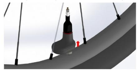
6. Tighten the TPMS and the adaptor simultaneously via tightening "The Adaptor".
