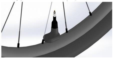
8. Check both the TPMS and adaptor can no longer rotate or wobble easily, the assembly is then complete.
