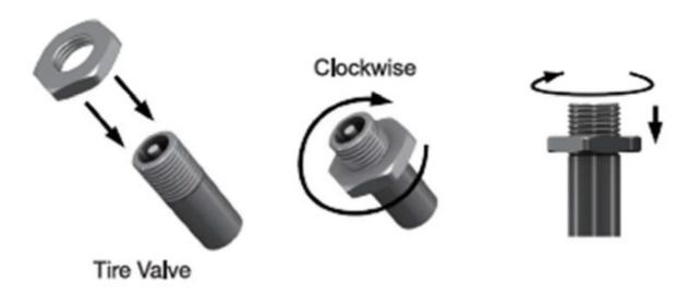
**Step 2**Lock sensor into valve, during lock-in process, you will hear the tire pressure leakage sound. Lock the sensor until no hearing tire pressure leakage sound to make sure sensor tightly locked.
