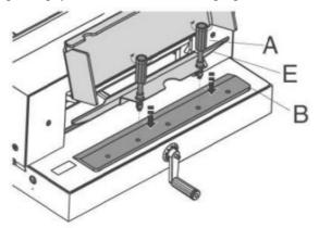
• Place the new blade A into the blade carrier D using the blade changing tool and push it up to the top screwing it using the grips B, fit three screws C with twe washers E and F screwing on blade carrier tightly using special too wrench and attachable extension pipe.
