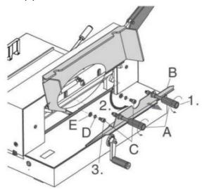
• Loosen two grips A to take out the blade changing tool B, fit two screws C with two washers D and E screwing on blade carrier tightly using special tool wrench and attachable extension pipe.
