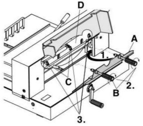
• Lightly tighten new blade B using two grips A on the blade changing tool E.
