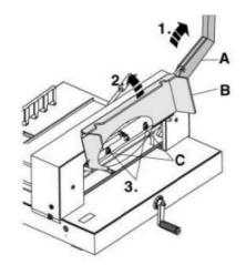
• Attach the blade changing tool A and screw tightly by two grips B then remove the other two screws C on the blade carrier using special tool wrench and attachable extension pipe.
