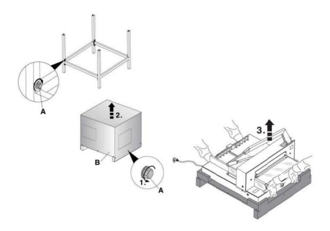
Place the guillotine correctly onto the machine stand. Tighten the four hecagonal nus with washers.
