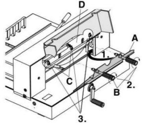
• Lightly turn two grips A on the blade charging tool anti- clockwise, take out blade carefully, put into the blade box C and tighten the blade in the box with two screws D
