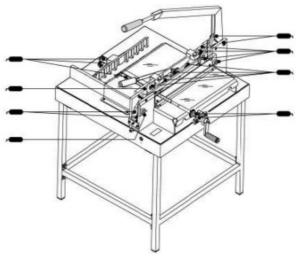
• The blade lever A should never fall automatically. If necessary tighten the hexagonal screw which can be accessed by removing the cover C.
