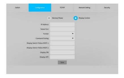
When there is a display (such as touch panel) connecting with two host sources and under the same network with the SCT-SW21UCKVM, we can control the display via the TCP/IP command setting.
