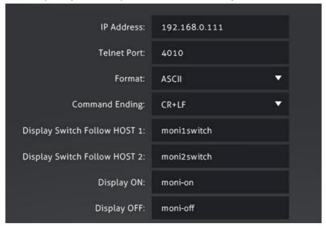
The SCT-SW21UCKVM will send the command moni-on to the TV when you send the command keypress:2 to the SW21UCKVM via the Crestron Controller.
