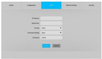
Send the TCP/IP command to other devices which is under the same network as SCTSW21UCKVM.
