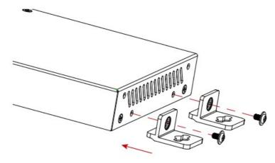
2. Install the brackets on the position as desired using screws (not included).
