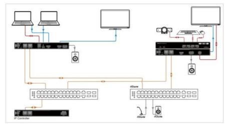
In this application, LAN1 (POE+) port is for transmission of A/V streams and control data; LAN2 is for transmission of Dante audio streams which is routed to a standalone network. Two Ethernet ports are connected to different networks.
