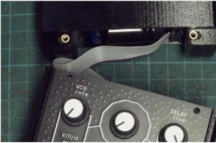
Now secure the front panel, rear and front part of the enclosure using 2x 12mm screws **(1)**, then using 2x 6mm screws **(2)**, fix the front panel to the front part.
