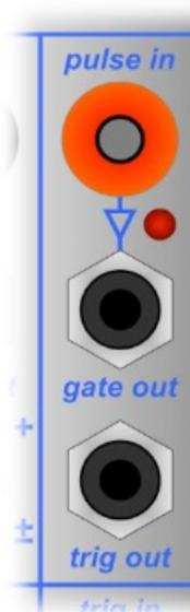
**pulse in** A 4mm banana socket input compatible with Buchla™ pulse outputs in the range of 0V to +15V.
