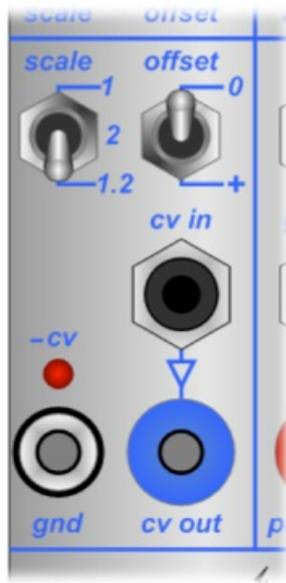
**cv in** A 3.5mm jack socket input from a Eurorack synthesizer
