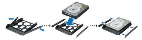
• For 2.5" drives: Remove the fastening panels from the sides of the drive tray and put them in a safe place. Place the drive in the blue area (shown below) of the drive tray, turn the tray upside down, and then tighten the screws provided to secure the drive.
