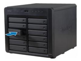
2 Pull the drive tray handle in the direction as indicated below to remove the drive tray.
