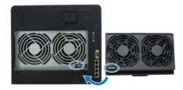
**b** Make sure that all 6 push pins on the new module are pulled outwards before the module is placed into your DiskStation, and then press the push pins back into place to secure the fan module.
