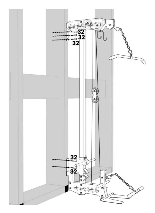
At your own deaccession the included wood screws to mount the pulldown machine to the center of a wall stud. Ensure the machine makes contact with the ground.
