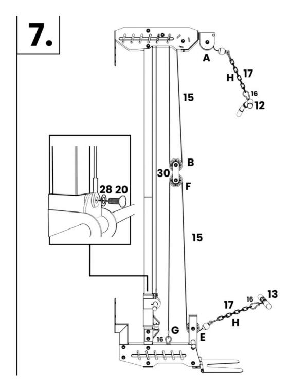
Follow the steps below to the corresponding letter to attach the cable to the pulley systems.
