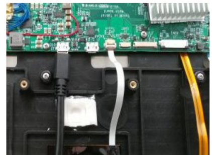
Figure 3-9: Touch cap FPC to PCB
