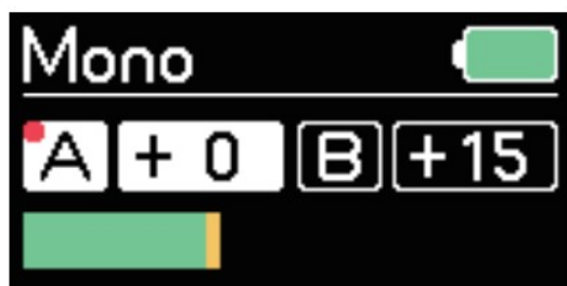
Red point on RX is flashing: Storage is full
