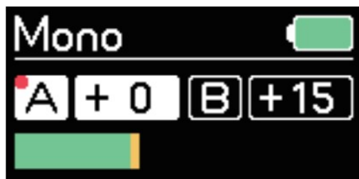
Red point on the RX's screen: Internal storage recording on
