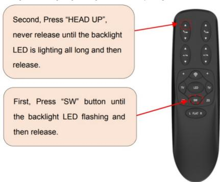
• When the Pairing Button/Program Button on the control box and the backlight LED on the remote stop flashing, and the buzzer on the control box has a "DI" sound, pairing is completed.
