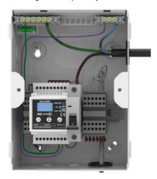
8. Terminate a twisted pair cable to the output terminals;s, these can be looped in/out of each charger, or multiple connections can be terminated into the Balancer. Ensuring correct polarity in the hub and the chargers.
