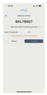
8. Check that the shown electrical measurements match the measurements. This will allow checking that the Load Management CT is fitted in the correct orientation and location. A negative value indicates a reverse direction of power due to to, e.g., solar surplus, but could also indicate that the clamp has been installed in a reversed (incorrect) orientation or polarity.
