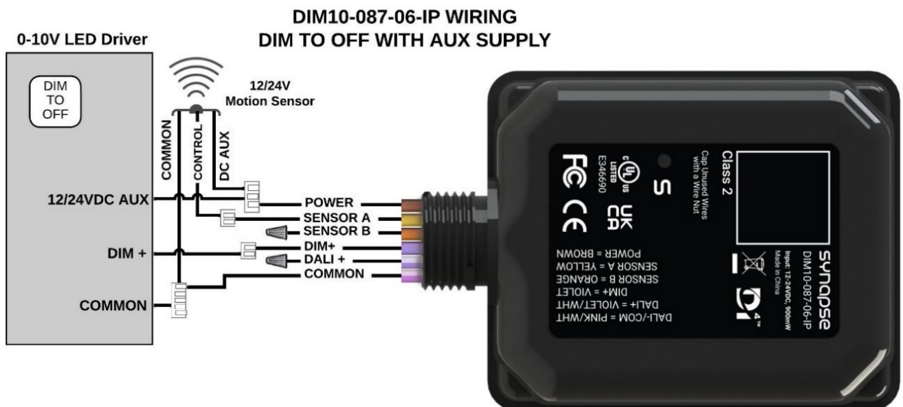
Figure 2 – D4i Wiring Diagram
