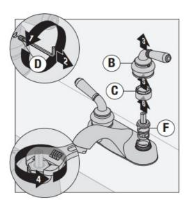
2) Correctly align new cartridge (E or F) and insert into faucet body (G). Install and secure nut (C).
