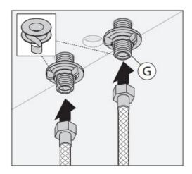
5) Attach supply lines to shut-off valves and hand tighten. Using a wrench, finish with one-half turn. **DO NOT** overtighten.
