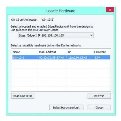
The Locate Hardware dialog will scan the selected Radius, Prism, or Edge unit and list xIn or xOut 12 units. Select the physical xIn or xOut 12 unit you wish to use and click the Select Hardware Unit button.
