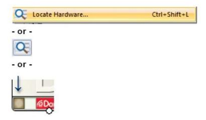
Discovery of, and connection to, Prism 4×4 hardware is done with the Locate Hardware dialog found under the Hardware menu or by clicking the Locate Hardware icon in the tool bar or on a particular Prism 4×4 unit itself.
