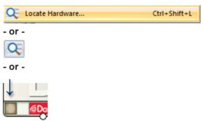
Discovery of, and connection to, Control Server hardware is done with the Locate Hardware dialog found under the Hardware menu or by clicking the Locate Hardware icon in the toolbar or on a particular Control Server unit itself.
