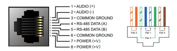
**Note:** The ARC Audio line may be grounded at the Symetrix rack-mount device and the ARC wall panel to provide additional distance.
