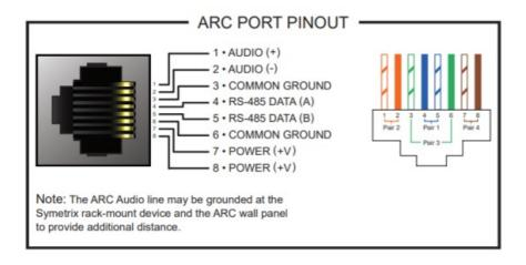
The Symetrix ARC-PSe provides serial control and power distribution over standard CAT5/6 cable for systems with more than 4 ARCs, or when any number of ARCs are located long distances from an Integrator Series, Jupiter or Symetrix DSP unit.
