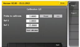
**Page 2:** allows a linearity correction using 2 to 25 points. The number of points and the measurement step can be entered. The value of the calibration blocks can be modified during the calibration procedure if it does not correspond to the measurement step.
