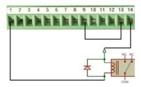
Note: a protective diode must be added in parallel of the relay if it isn't integrated.
