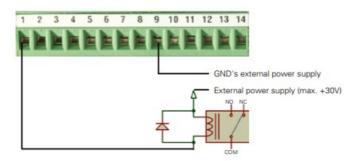
Note: a protective diode must be added in parallel of the relay if it isn't integrated.
