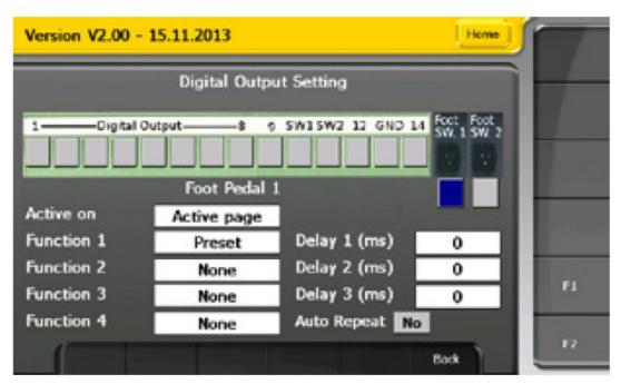
Function: Pedal function configuration. Up to 4 different functions can be combined. A delay between each of the functions can be defined in milliseconds.
