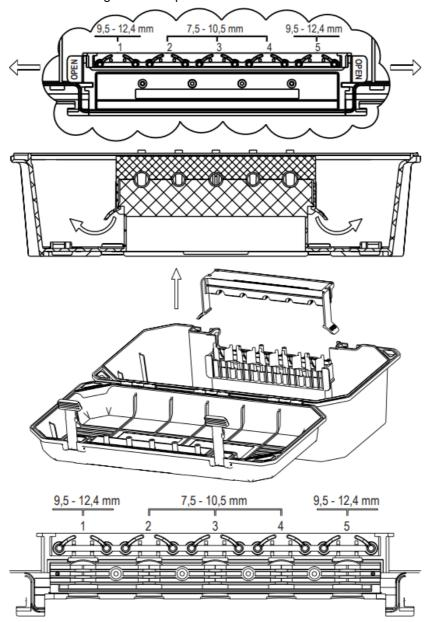
7.3 Lay the cables and reassemble the clamps
