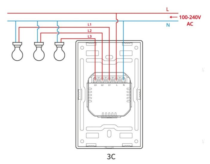
3. \*To ensure the safety of your electrical installation, it's essential either a Miniature Circuit Breaker (MCB) or a Residual Current Operated Circuit Breaker (RCBO) with an electrical rating of 10A 1C,2C),6A 3C)has been installed before the M5-120W.
