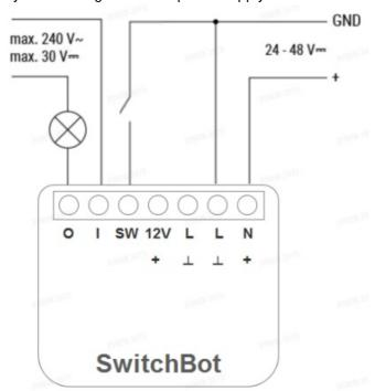
The voltage on the I and O terminals of the Device should not exceed 30V.
