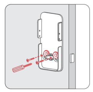
Step 4: Install the cylinder adaptor.
