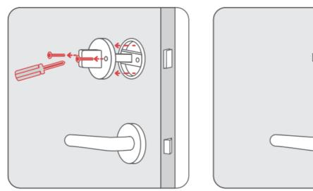
Step 3: Install the mounting bracket
