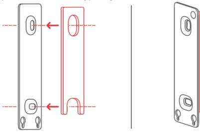
Step 3: Attach Keypad to Mounting Plate
