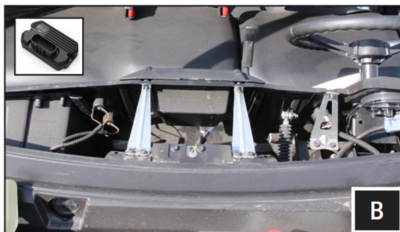
B. Lift and gently pull the dash cover away from the vehicle to expose the dash cavity. Locate a suitable mounting location for the TANGO2 Turn Signal module. Secure the module to a panel using screws or zip tie it to a harness.
