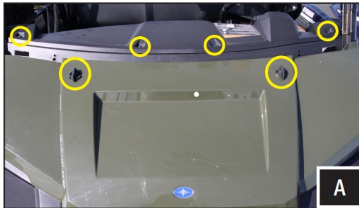
A. Using a panel tool, remove the (4) push pins retaining the dash cover.
