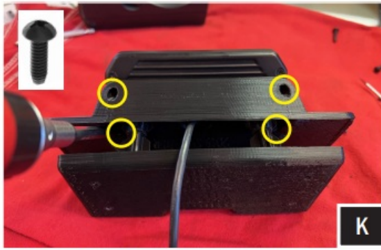
K. Use (4) 4-40x.375 Thread Cutting screws [B-S3262] to secure the 15-button controller to the Sprinter ALPHA12 overhead mounting kit.
