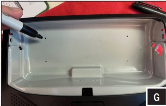
G. Use a marker to emphasize the screw hole points.
