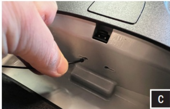
C. Unhook the (2) rubber limiter bands in the sunglass holder.
