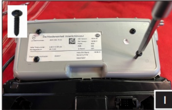
I. Hold the Sprinter mounting bracket in the sunglass holder cavity while fastening the back side with (4) #7-19 screws (B-S1656).
