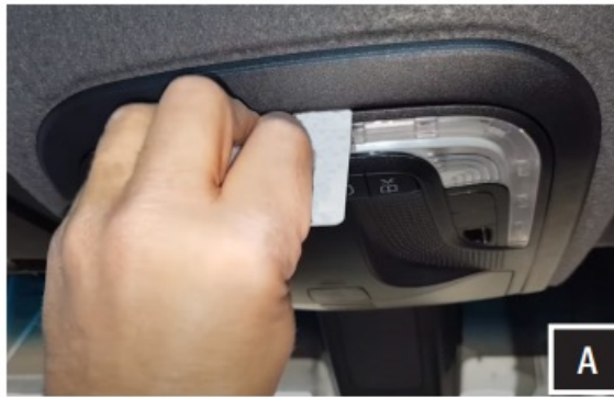
A. Insert a credit card in the middle front side of the overhead console to release the lock and slide out the overhead console.
