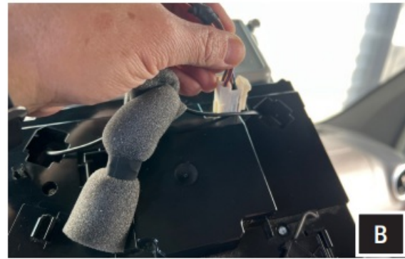
B. Unplug the connectors behind the overhead console.
