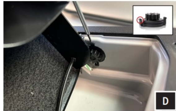
D. Remove the plastic rotary damper by carefully pressing on the lock.
