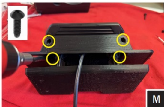
M. Use (4) 4-40x.375 Thread Cutting screws [B-S3262] to secure the 15-button controller to the Sprinter ALPHA12 overhead mounting kit.
