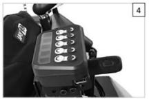
4. The CTRL+5 has a built-in USB port for charging or powering peripheral devices (Fig. 5). The current is limited to 2.0 Amps, which is sufficient to charge most smartphones and tablets.
