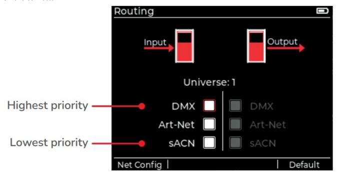
Either the Input or Output side will be active, depending on which app is being used: Receive or Send For Art-Net and sACN signals, use the keys to choose the required universe
