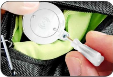
3. Separate the FMN device from the bracket
