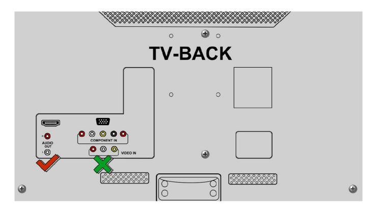
**Step 2:** Use the 3.5 mm audio cable connect the RCA aux converter cable that we provided, and then connect your TV to the adpater (In TX mode), then turn on the Bluetooth headset and put it together. After the pairing is successful, you should be able to hear your TV through the headset.
