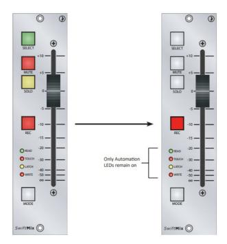
A few seconds after initial power up, the SELECT, MUTE, SOLO, and REC LEDs should turn off. The READ, TOUCH, LATCH, and WRITE automation mode LEDs should remain illuminated. At this point, the SwiftMix<sup>™</sup> faders are in DAW select mode.
