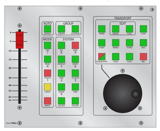
**LOOP** – Pressing this button toggles Loop Playback mode on and off.
