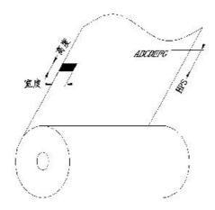
Printing position: As shown in the figure above, the black mark should be printed on the left edge of the non-text side.
