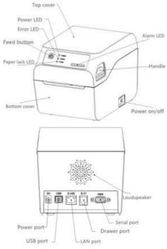
Figure 2-1 The name of each part of the printer
