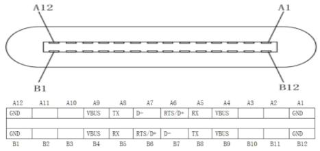
USB TO Type-C Socket and PIN Assignment
