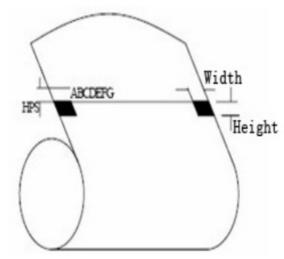
Printing Position: As the picture above, the black mark should be printed on the right edge of the printed side of paper.
