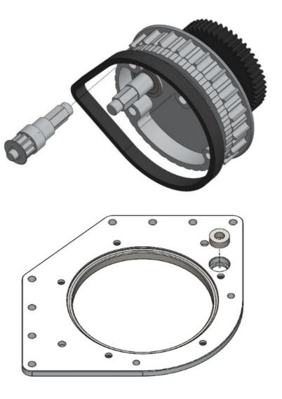
Insert Base Pulley Assembly, aligning Base Pulley with X-Contact Bearing and Steering Shaft with R188ZZ Bearing. Insert 15t Bevel Gear, followed by .5mm Shim and 688 Bearing.
